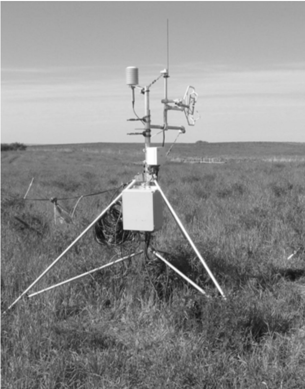
Figure 2. Eddy covariance system and land surface vegetation at St Denis National Wildlife Area
