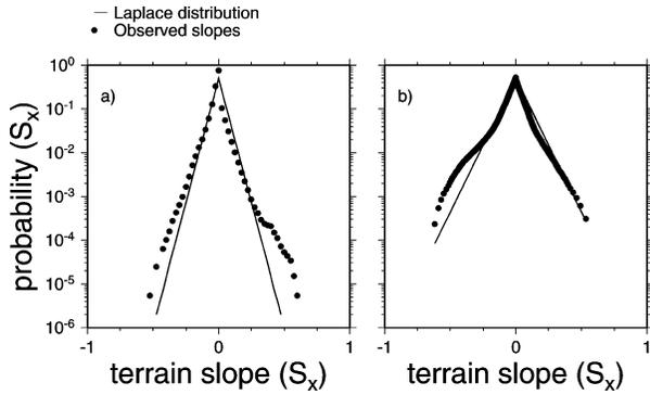
FIG. 3. Laplace distribution fit to east–west terrain slopes for (a) Trail Valley Creek and (b) Innavaik Creek.
