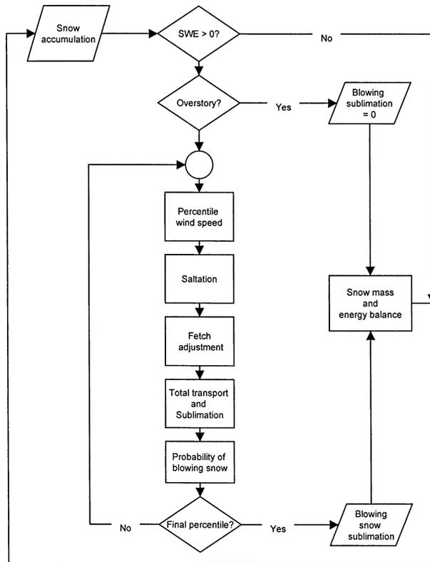
FIG. 2. Schematic illustrating the calculation of sublimation from blowing snow and interaction with the existing VIC snow model.
