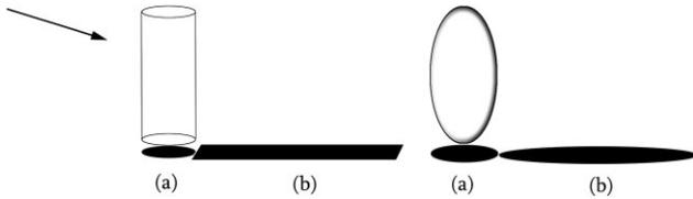
Figure 5. Illustration of the (a) non-overlapping ( $x_{NO}$ ) and (b) overlapping ( $x_O$ ) components of trunk (left) and crown (right) shadows projected upon a horizontal surface by their respective geometric shapes. Arrow indicates direction of incident shortwave ray
