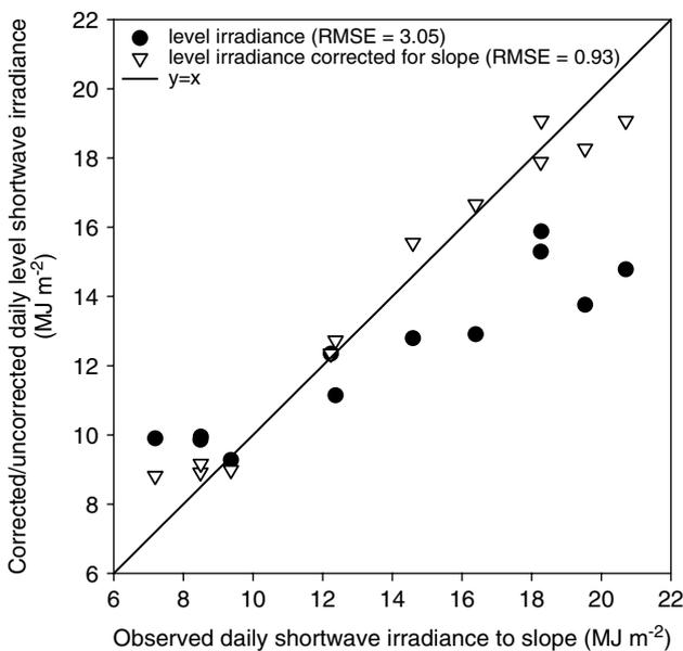
Figure 3. Scatterplot comparing observed daily shortwave irradiance to a slope of 27° slope gradient, 128° azimuth to corrected/uncorrected irradiance to a nearby level surface. RMSE is in  $\text{MJ m}^{-2} \text{d}^{-1}$
