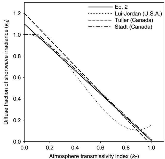
Figure 4. Correlations of diffuse shortwave irradiance fraction ( $k_d$ ) to atmospheric transmissivity index ( $k_T$ ) developed from measurements in Canada (Tuller, 1976; Stadt *et al.*, 2005) and the United States (Lui and Jordan, 1960) compared to Equation (2)
