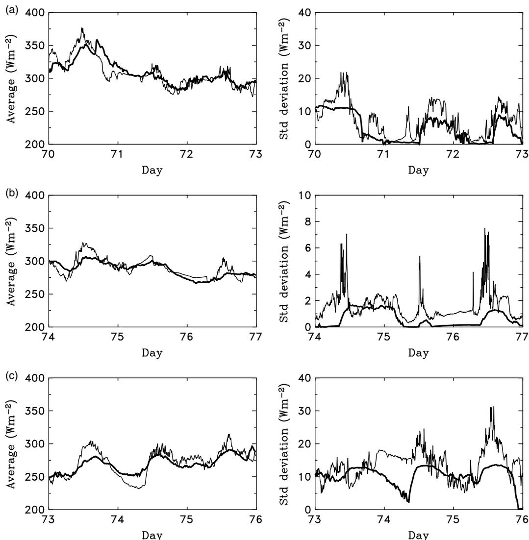
Figure 6. As Figure 5, but for the model using measured sky view and air temperature and modelled above-canopy longwave radiation
