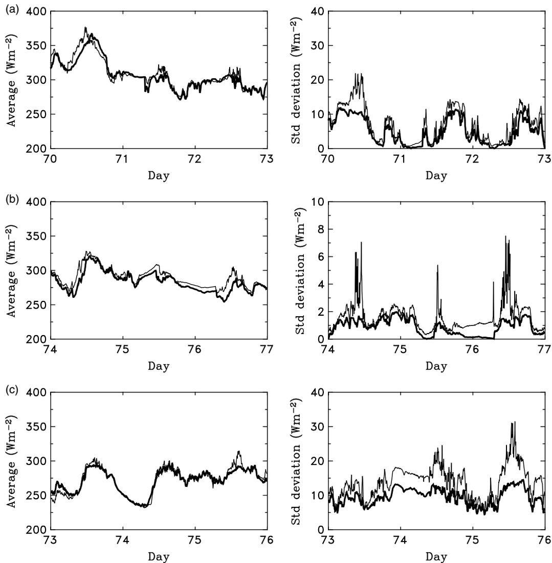
Figure 5. Spatial averages (left) and standard deviations (right) across the radiometer arrays for (a) the southeast-facing forest, (b) the level forest and (c) the forest gap. Thin lines are from measurements and thick lines are from the model using measured sky view, air temperature and above-canopy longwave radiation
