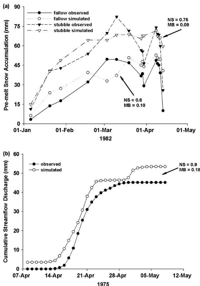
Figure 4. CRHM test: (a) simulated pre-melt snow accumulation and observed pre-melt snow accumulation in fallow and stubble fields of Bad Lake Research Basin during the winter of 1981–1982, (b) simulated cumulative streamflow discharge during snowmelt and observed streamflow discharge for Creighton Tributary, spring 1975
