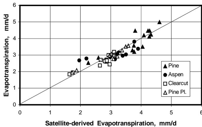
**Figure 2** Comparison of daily evapotranspiration values obtained using a conventional model in conjunction with ground-based data with those obtained using satellite-derived data.
