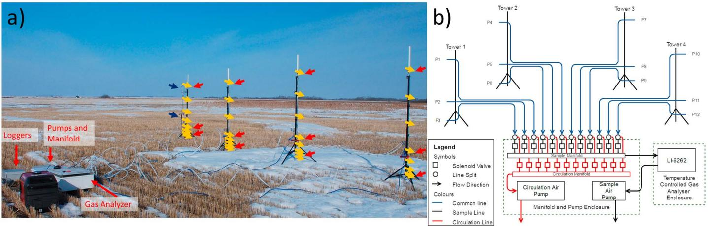
**Figure 1.** (a) Deployed atmospheric profile observation system. Sensors are spread over 4 mobile towers and include 2 three-cup anemometers (blue arrows), 32 fine wire thermocouples (yellow arrows) and 12 water vapor intakes (red arrows) that (b) are routed sequentially to a common gas analyzer.
