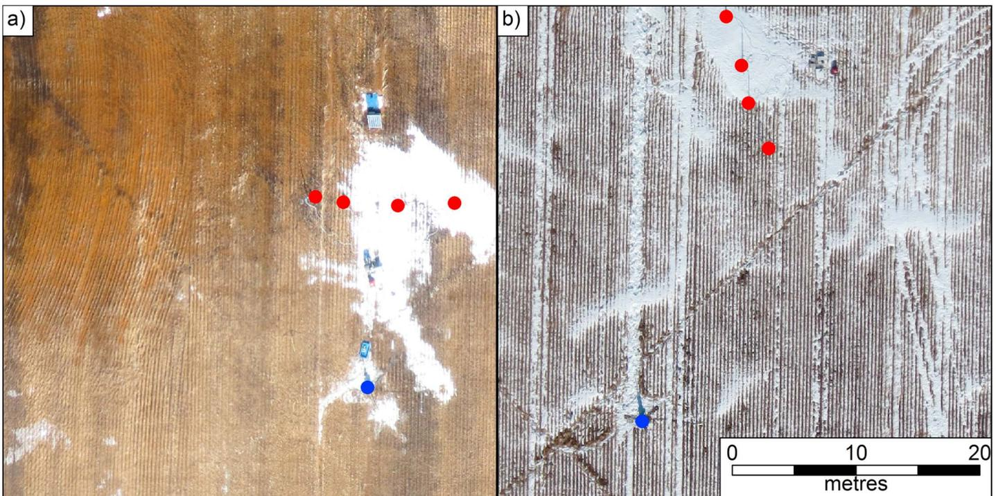
**Figure 2.** Unmanned aerial vehicle imagery of (a) 18 March 2015 and (b) 30 March 2015 deployments. Red points are locations of towers with Tower 1 upwind in nonsnow location, Tower 2 located at transition, and Towers 3 and 4 situated sequentially downwind over snow. Towers are in line with the prevailing wind direction over the observation interval. Blue dot is location of eddy covariance system and additional in-field instrumentation.
