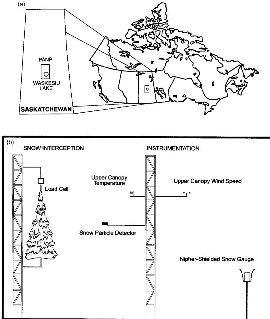
Figure 1. (a) Experimental site location. (b) Tower design and instrumentation. The schematic conceptualizes the basis for the towers used at the jack pine and black spruce sites
