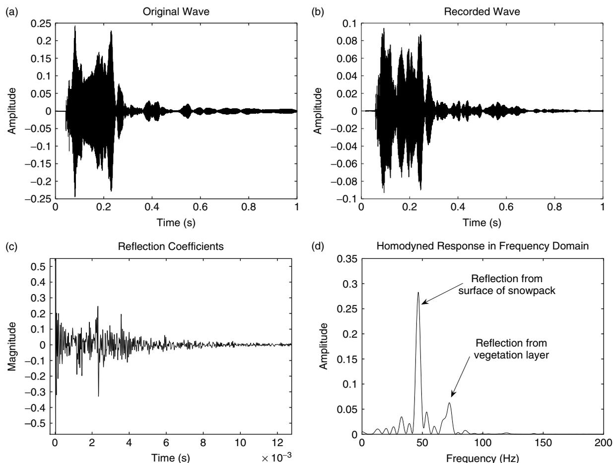
Figure 8. Signals in the time and frequency domains for the  $N = 1$  layered snowpack. (a) original wave, (b) recorded wave, (c) reflection coefficients, (d) homodyned response in frequency domain. The amplitudes of Figure 8(a), (b), and (d) are normalized. The beat frequency  $\Delta F_{b,k}$  is given in Figure 8(d)
