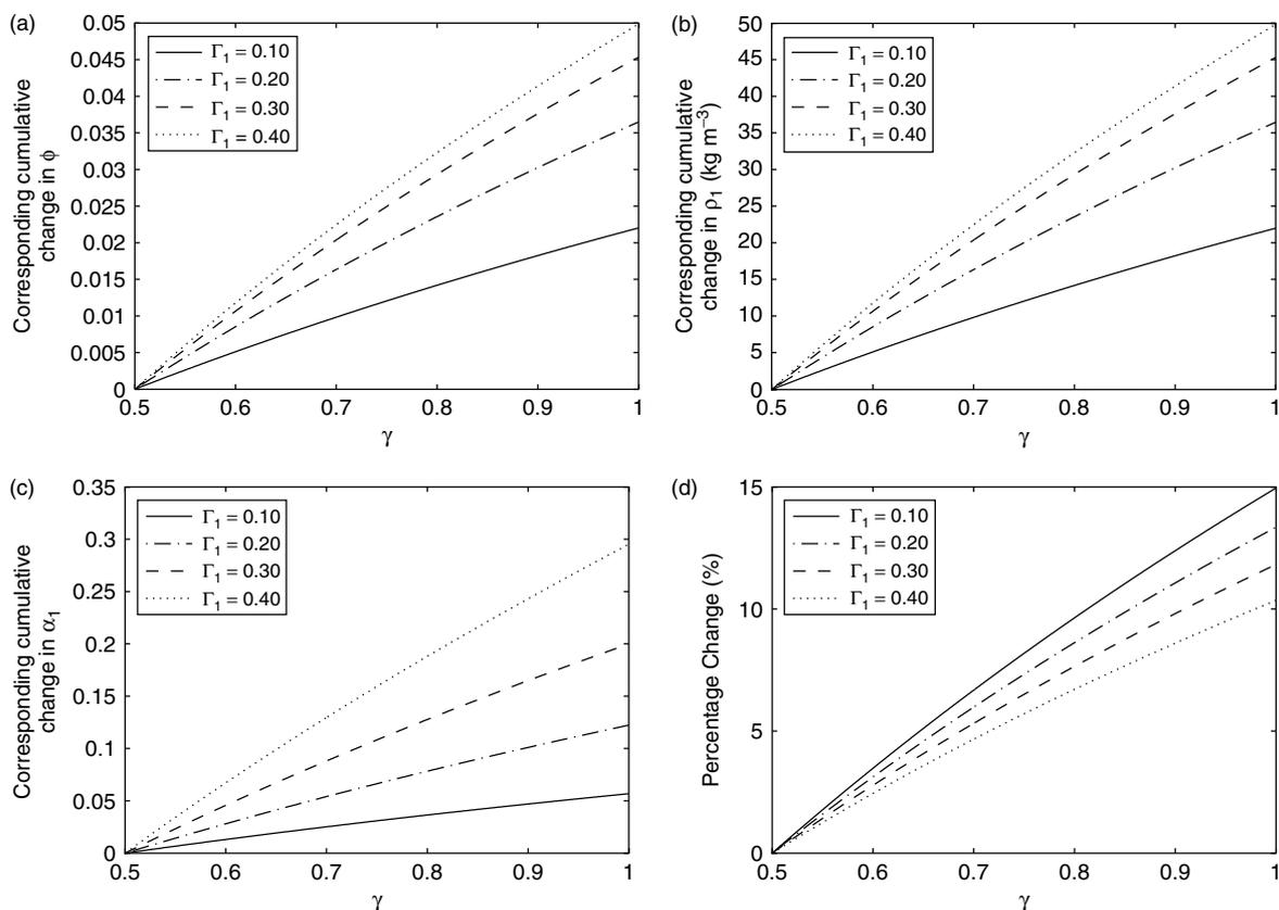
Figure 12. Sensitivity analysis for the air-snow interface. (a) Examining sensitivity of  $\phi$  to change in shape factor  $\gamma$ ; (b) Examining sensitivity of  $\rho_1$  to change in shape factor  $\gamma$ ; (c) Examining sensitivity of  $\alpha_1$  to change in shape factor  $\gamma$ ; (d) Percentage difference of  $\rho_1$  due to change in shape factor  $\gamma$
