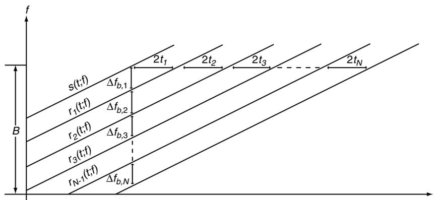
Figure 5. Conceptual diagram of the snowpack response. The signal that is transmitted from the speaker is  $s[t, f]$ . The reflected signals  $r_1[t, f], \dots, r_N[t, f]$  from each of the layers in the snowpack are shifted in frequency by  $\Delta f_{b,k}$  for the  $k$ th layer of the snowpack system
