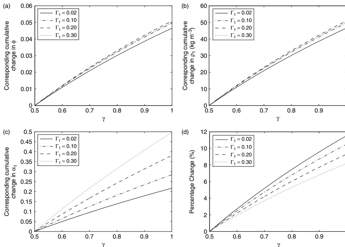
Figure 13. Sensitivity analysis of the snow-snow interface. (a) Examining sensitivity of  $\phi$  to change in shape factor  $\gamma$ ; (b) Examining sensitivity of  $\rho_1$  to change in shape factor  $\gamma$ ; (c) Examining sensitivity of  $\alpha_1$  to change in shape factor  $\gamma$ ; (d) Percentage difference of  $\rho_1$  due to change in shape factor  $\gamma$
