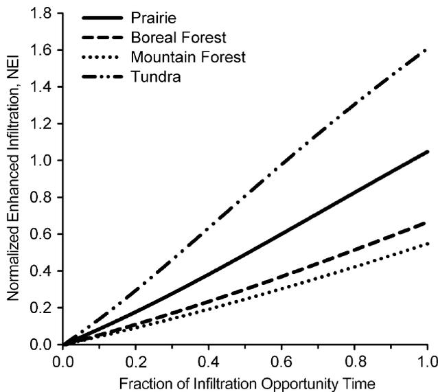
Figure 6. Variations in normalized enhanced infiltration at four demonstration sites over the course of the melt
