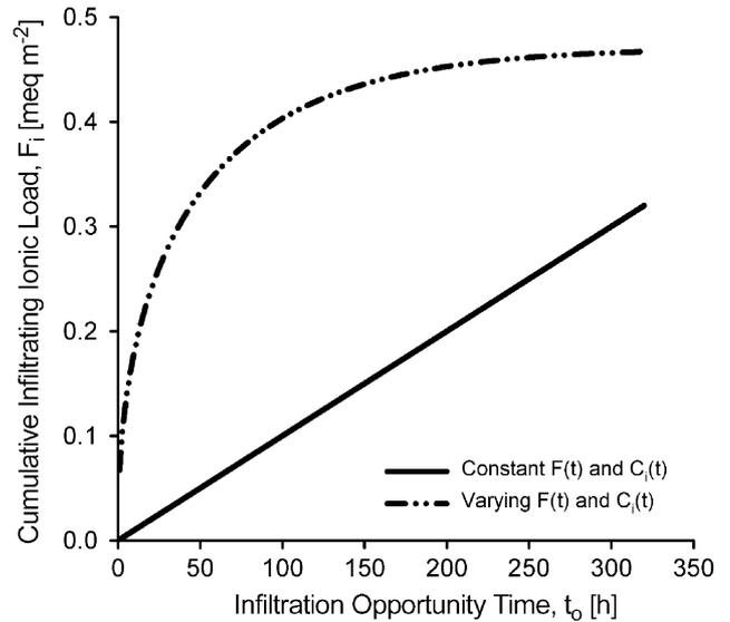
Figure 2. The cumulative load of an ion that infiltrates frozen soil if infiltration rate,  $f(t)$ , and ion concentration,  $C_i(t)$ , are held constant with time and if both parameters vary with time respectively
