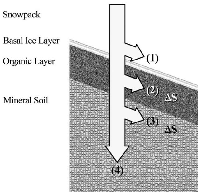
Figure 1. Below a melting snowpack, meltwater is partitioned into (1) ponded water, basal ice storage, and overland flow, (2) organic layer storage and interflow, (3) infiltration to frozen mineral soils with subsequent storage or interflow, and (4) percolation to groundwater
