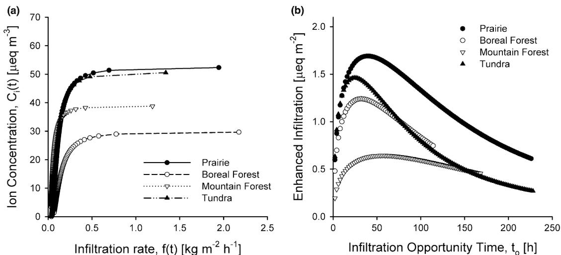
Figure 5. (a) The relationship between infiltration rate,  $f(t)$ , and ion concentration,  $C_i(t)$ . (b) Variation in enhanced infiltration of ions over the snowmelt period
