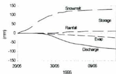
Figure 2a: Cumulative water balance components for Trail Valley Creek for the 1996 snowmelt period.
