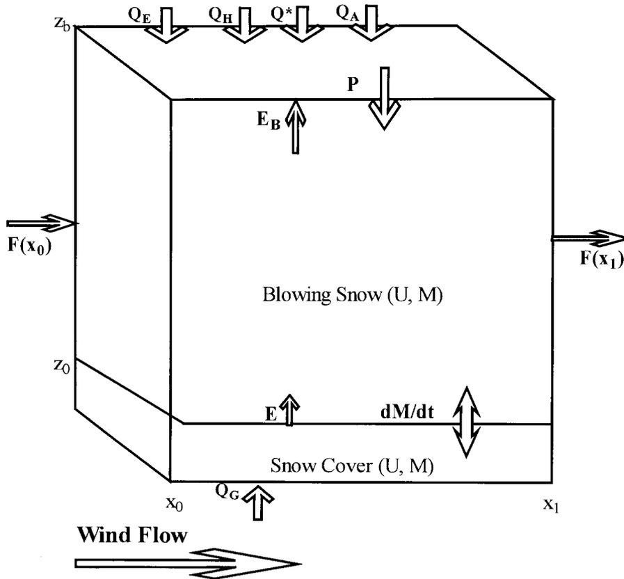
Figure 1. Control volume of blowing and surface snow with energy and mass fluxes indicated
