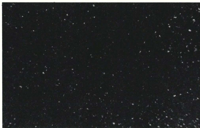
Fig. 1. Photograph of blowing-snow particles sampled at 1 m height. The width of the sample is 50 mm. Atmospheric conditions: air temperature -12^\circ\text{C} , relative humidity 62%, wind speed at 1 m height 11 m/s; time and place 13.00 h, 12 February 1985.
