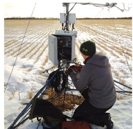
Measuring atmospheric energy for snowmelt and melt rates in a cultivated field near Rosthern, Saskatchewan
