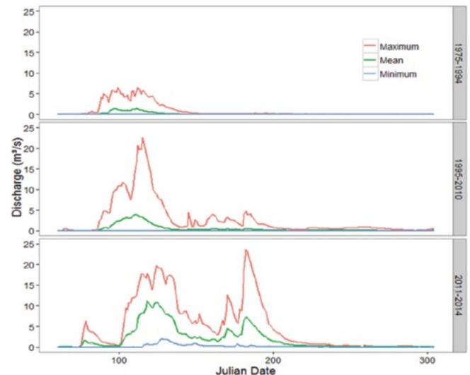
The changing hydrology of Smith Creek, Saskatchewan. Streamflow discharge measurements from January 1<sup>st</sup> show a dramatic change from 1975 to 2014.
