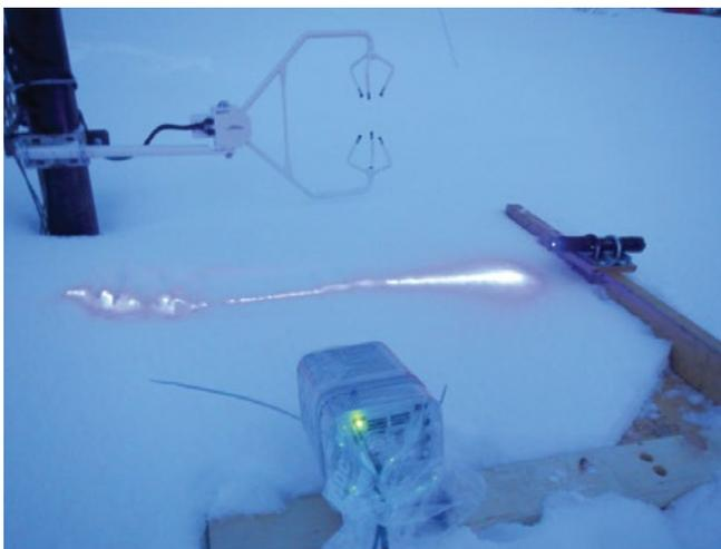
Laser-based measurement of blowing snow using high speed photography to track individual blowing snow particles as they cross a field.
