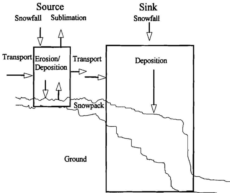
Figure 1. Arctic Blowing Snow Model. Schematic showing fluxes and mass balance over an irregular landscape.
