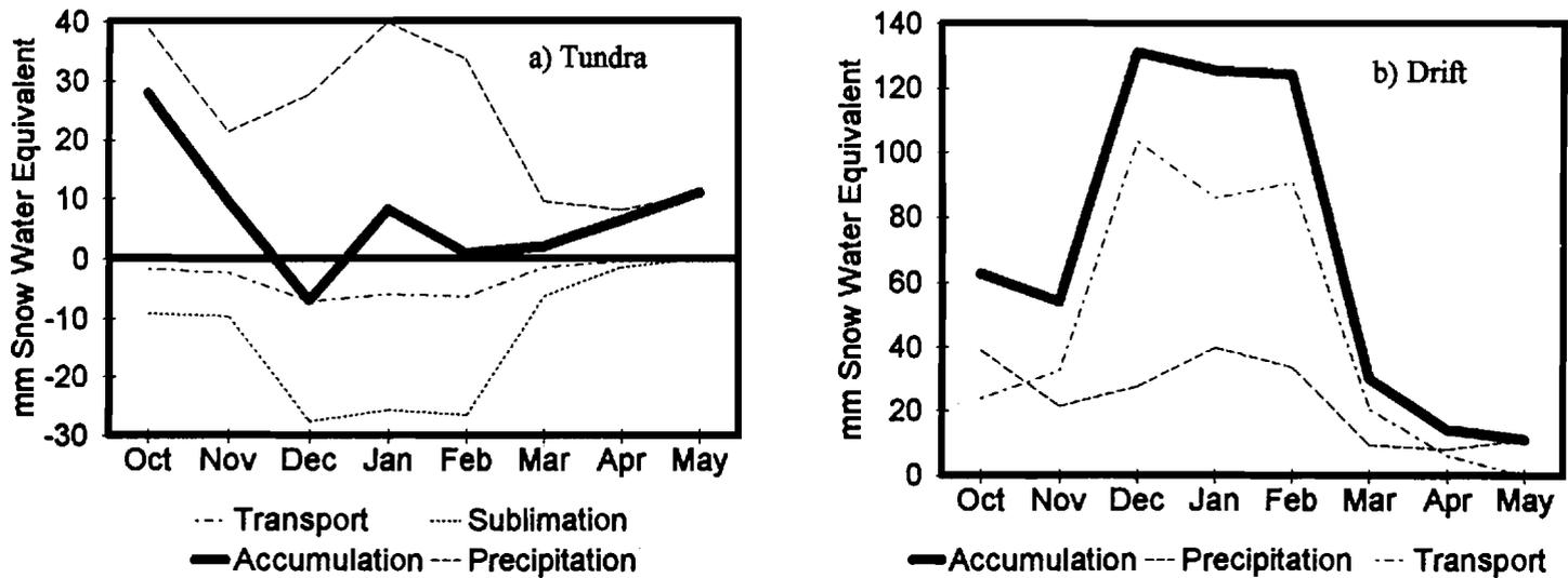
Figure 2. Monthly snow fluxes on surfaces of Tundra (a) and Drift (b) at Trail Valley Creek, NWT for 1992-93 as predicted by the ABSM.
