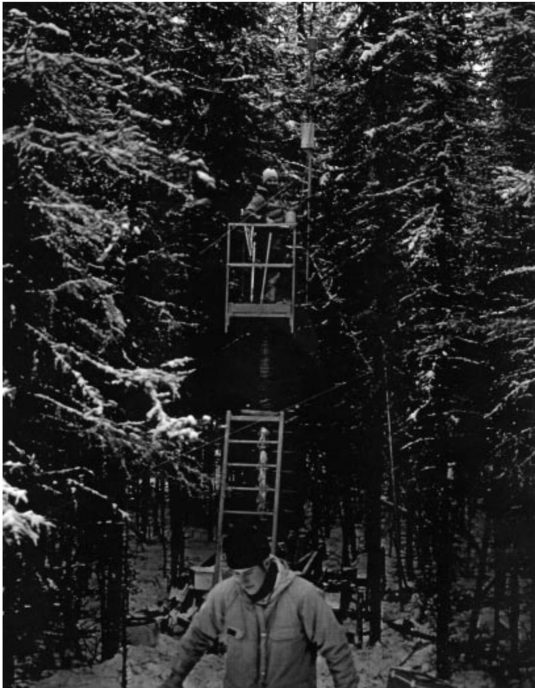
Figure 2. Photograph of portable elevator and sampling method used to obtain intercepted snow samples in a black spruce stand. Note that the elevator is only extended during sampling so that the intercepted snow is otherwise undisturbed
