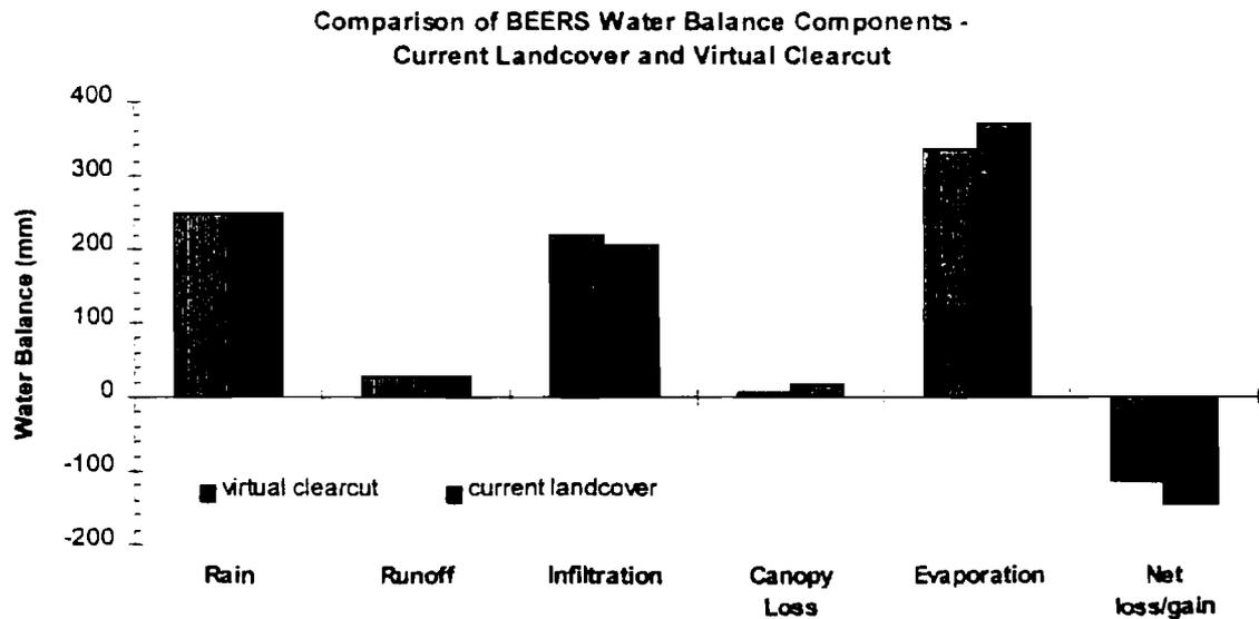
Figure 12. Comparison of modelled summer water balance for undisturbed and virtual clear-cut of conifer stands in Beartrap Creek basin, 1995.
