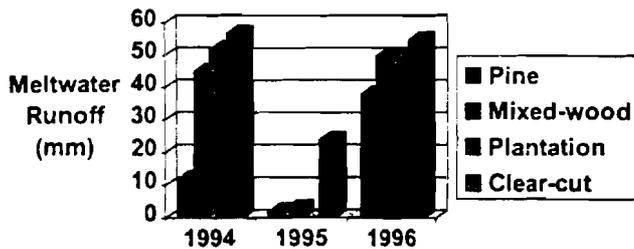
Figure 9. Snowmelt runoff from forest stands as a function of forest cover. The clear-cut consistently produces more runoff than do the undisturbed forest sites.
