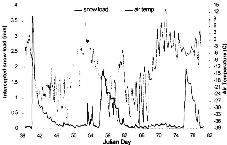
Figure 4. Sequence of snow interception and sublimation measured from a suspended jack pine tree. Snow mass on the tree has been converted to areal snow water equivalent by comparing changes to tree mass during snowfall to a mass balance of above and below canopy snowfall. Air temperature is also shown to indicate that it is sublimation rather than melt which reduces most intercepted snow in this environment.
