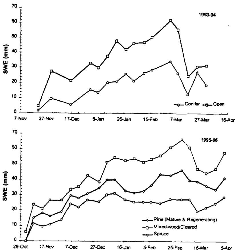
Figure 6. Seasonal time series of snow water equivalent accumulation under various canopy types. Snow accumulation decreases with increasing leaf area because of interception and subsequent sublimation losses.
