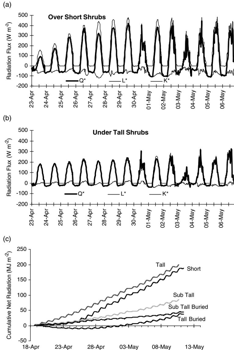
Figure 7. Net radiation  $Q^*$  and its components net longwave radiation  $L^*$  and net shortwave radiation  $K^*$  regimes. (a) *Over* short shrubs (which became snow free after 29 April); note that  $L^*$  is always slightly negative. (b) *Under* tall shrubs during snowmelt with increasing shrub exposure; note that  $L^*$  is always near zero. (c) Cumulative net radiation above and below tall shrubs, buried tall shrubs (mostly) and short shrubs during snowmelt
