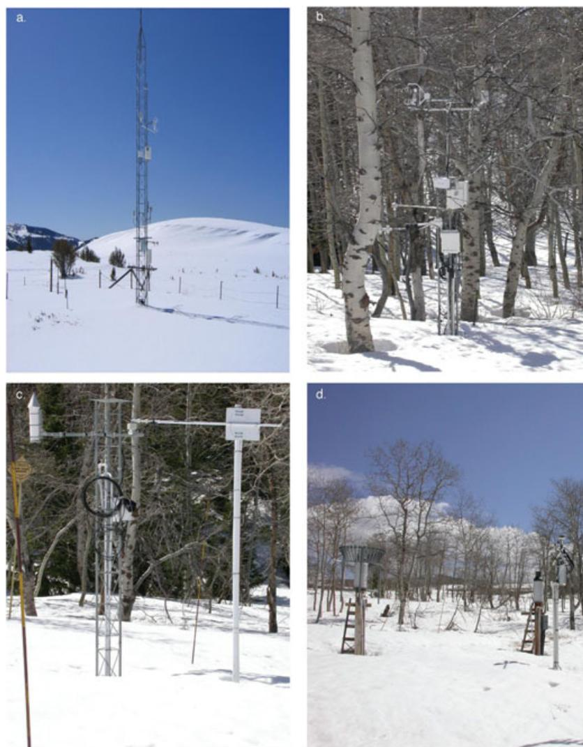
Figure 2. (a) An upwind view from the wind-exposed eddy covariance (EC) site, (b) the sheltered EC site, (c) an upwind view from the sheltered snow pillow site and (d) a downwind view from the sheltered snow pillow site. The sheltered EC site and sheltered snow pillow site are approximately 70 m apart
