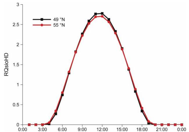
Figure 8 | Hourly values of  $R_{QsioHD}$  (the ratio of  $Q_{siH}$  to  $Q_{sioD}$ ), computed for latitudes 49° and 55°N, for day number 172 (June 21, for non-leap year).
