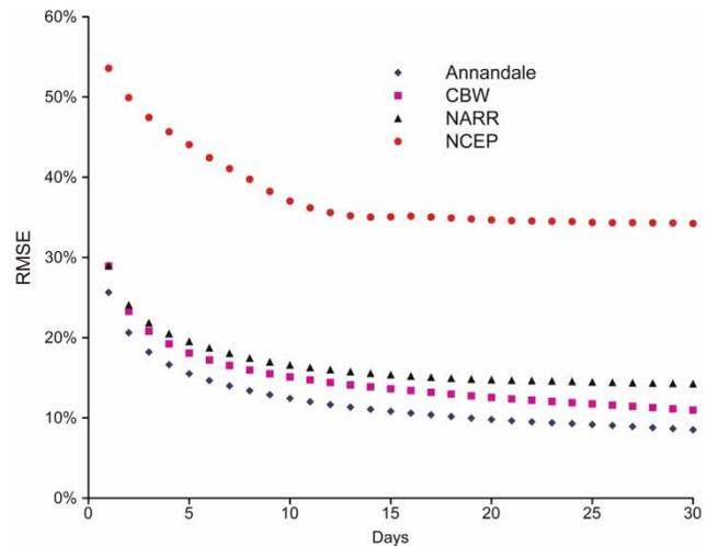
**Figure 5** | Mean total RMS error (percent) versus number of days for estimation of  $Q_{siD}$  during March and April.
