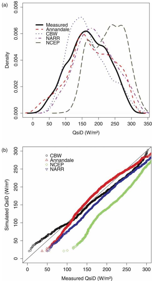
**Figure 6** | Plots describing frequency distributions of Edmonton measured and simulated  $Q_{siD}$ . (a) Kernel density plots of Edmonton spring measured, Annandale, CBW, NARR, and NCEP  $Q_{siD}$ . (b) Quantile-quantile plots of Edmonton spring Annandale, CBW, NARR, and NCEP  $Q_{siD}$ , against measured quantiles. The line is 1:1.
