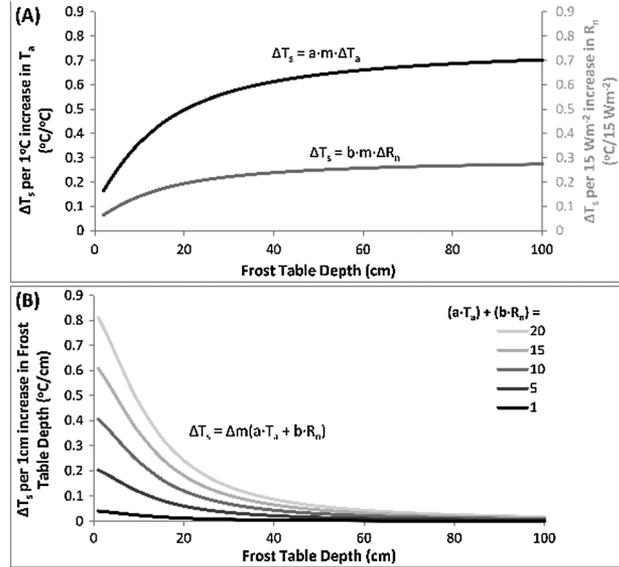
Figure 2. Sensitivity of variables in the RCC relation (with  $a=0.77$ ,  $b=0.02$ ) to (A) changes in air temperature and net radiation and (B) changes in frost table depth. In each case, the change in calculated ground surface temperature is based on the position of the frost table (x-axis)
