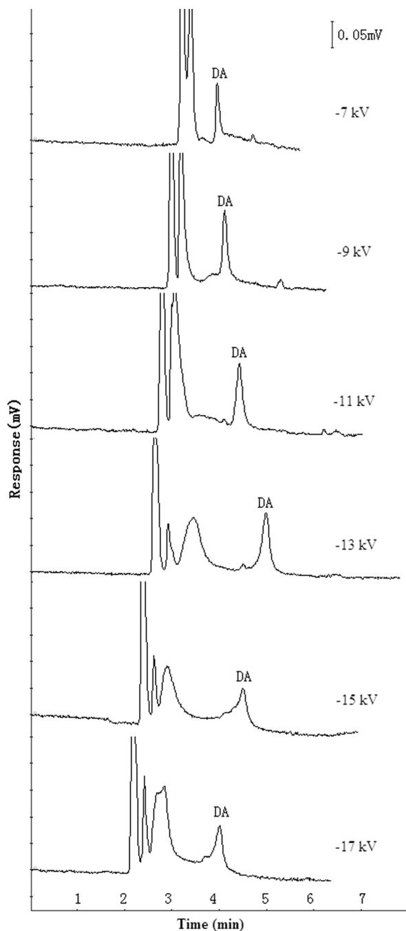
**Figure 2.** Effect of applied voltage on separation of mussel tissue extract spiked with 5 mg/L DA. Experimental conditions, mobile phase, 60% v/v ACN, 40% v/v of 5 mmol/L Tris buffer solution (pH = 8.0); supplementary pressure, 7.2 MPa; applied voltage as shown in this figure. Other conditions are the same as in Fig. 1.
