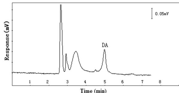
**Figure 3.** Typical electrochromatogram of mussel tissue extract spiked with 5 mg/L DA under the optimal conditions. Peaks before DA are of matrix solutes.
