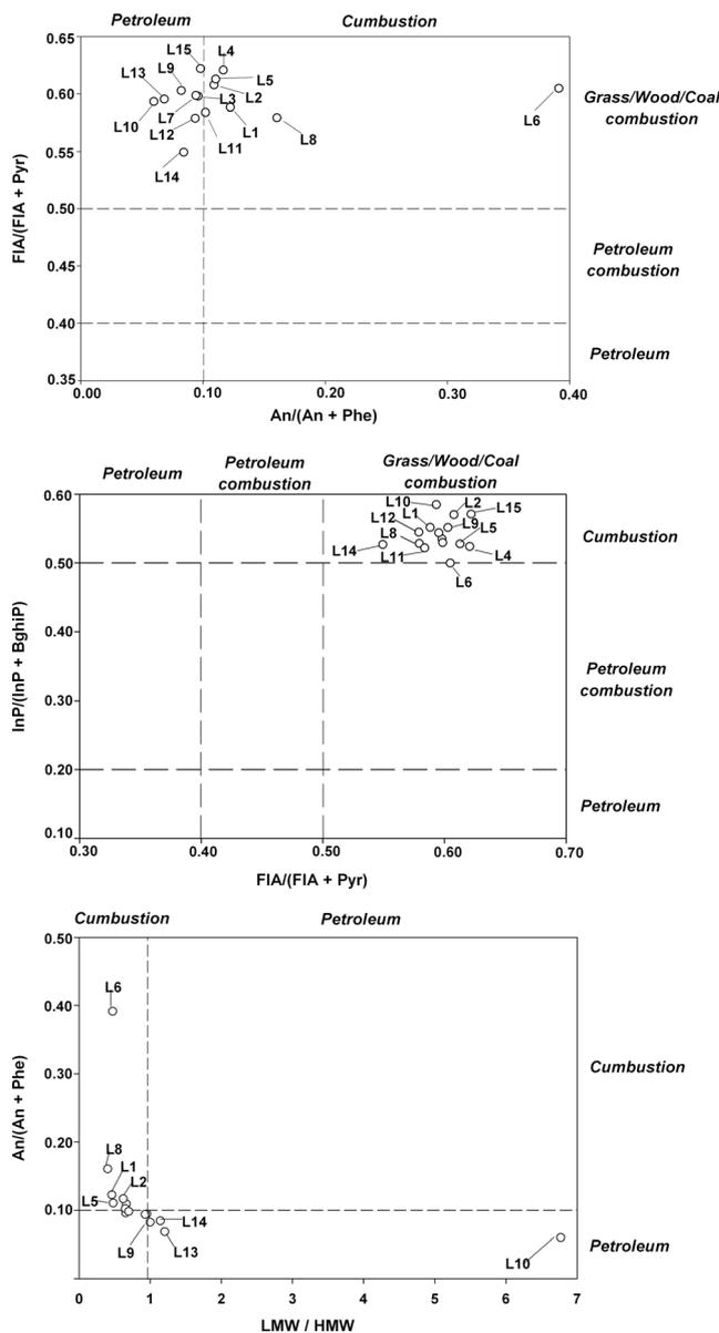
**Fig. 4** PAH cross-plots for the ratio An/(An + Phen) versus FIA/(FIA + Pyr) (a), FIA/(FIA + Pyr) versus InP/(InP + BghiP) (b), and LMW/GMW versus An/(An + Phen) (c)
