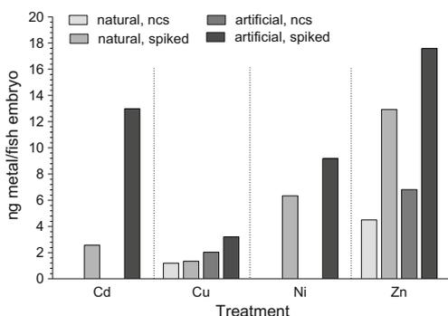
**Fig. 2** Metal concentrations in zebrafish embryos (ng/embryo) exposed to natural and artificial sediments spiked with a mixture of four metals over 48 h compared to unspiked control sediments (ncs=negative control sediment); columns represent individual measurements of single composite samples containing 50 (natural sediment) and 30 (artificial sediment) measured embryos per treatment (one replicate)
