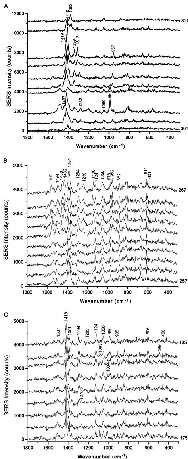
**Figure 6.** Selected SERS spectra recorded between time intervals as indicated (A from 301 to 311 s, B from 257 to 267 s, and C from 175 to 185 s). 6A shows strong intensity fluctuations while in 6B and 6C most bands have comparable intensities over several seconds. Integration time 1 s; background has been subtracted. Spectra are plotted on the same scale as indicated and are offset for clarity.
