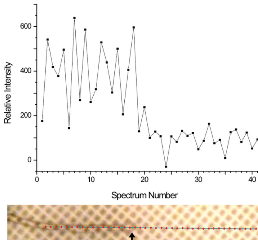
**Figure 3.** Representative line map of a fungal hypha with the intensity plot of the band at  $1050\text{ cm}^{-1}$ . The red points on the hypha image (bottom) indicate the measurement position and correlate with the squares in the intensity distribution profile (top). The single-headed arrow indicates the approximate tip of the fungal hypha between pixels 17 and 18.
