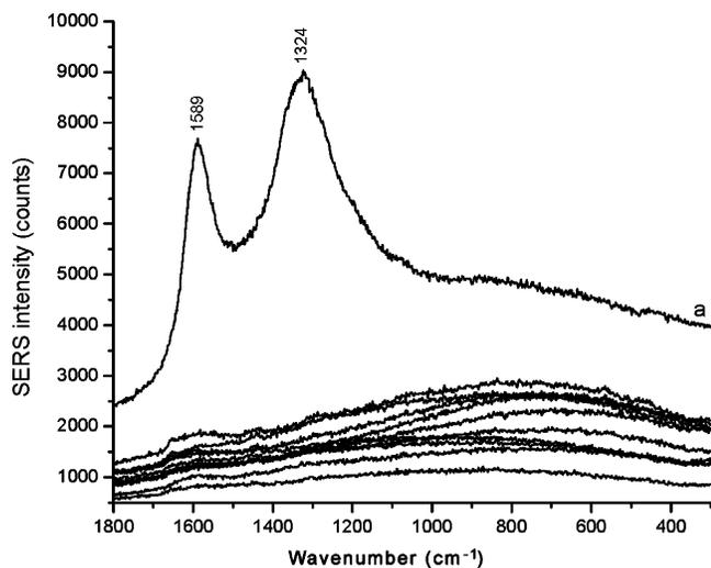
**Figure 8.** Selected SERS spectra recorded from gold substrate in absence of fungi ( $\sim 1\text{--}2$  mm from fungal tips). Integration time 1 s; spectra recorded in a row with  $1\ \mu\text{m}$  spatial resolution. Spectrum a shows characteristic amorphous carbon bands.
