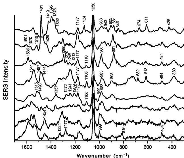
**Figure 7.** Average spectra of SERS time-dependent measurements recorded on hot spots with strong intensity fluctuations. A total of 90–300 SERS spectra obtained with 1–5 s integration time/spectrum were averaged.
