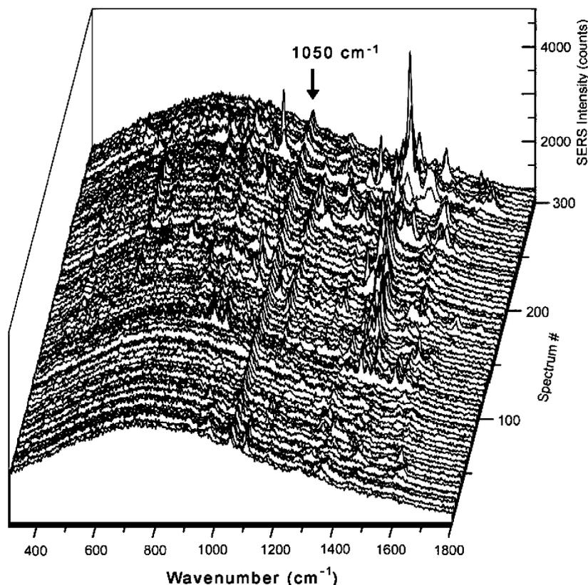
**Figure 4.** Time-dependent SERS spectra of *A. nidulans* recorded with 1 s integration time showing every fifth spectrum. The background has not been subtracted. Total measurement time was  $\sim 350$  s, and a total of 300 spectra were recorded.
