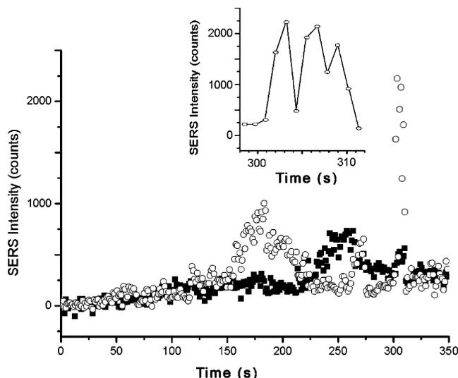
**Figure 5.** Plot of the SERS intensity of the spectra in Figure 4 for the peak positions at 611 (■) and 1419  $\text{cm}^{-1}$  (○) as function of time. The same background line has been subtracted from all 300 spectra. Insert shows an enlargement of the peak intensity at 1419  $\text{cm}^{-1}$  from  $\sim 300$  to 310 s with rapid intensity fluctuation. The insert shows the region from 300 to 310 s with the time scale expanded.
