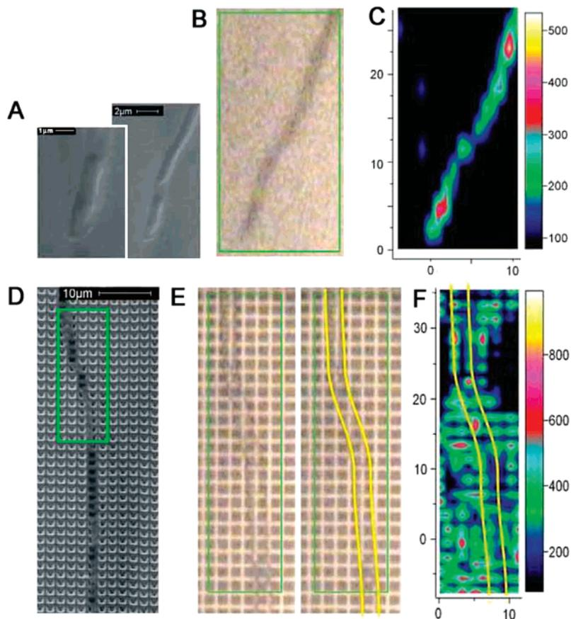
**Figure 2.** SEM (A, D) and photo images (B, E) of fungi grown over smooth gold surface and SERS active region, respectively. Raman (C) and SERS (F) spectral maps processed for the area of the band at  $1050\text{ cm}^{-1}$  for the regions outlined in the photoimages B and E. Spectral maps were measured at  $633\text{ nm}$  excitation with 180 s integration time for Raman and 10 s for SERS. Color bars show correspondence between band area and processed map colors.
