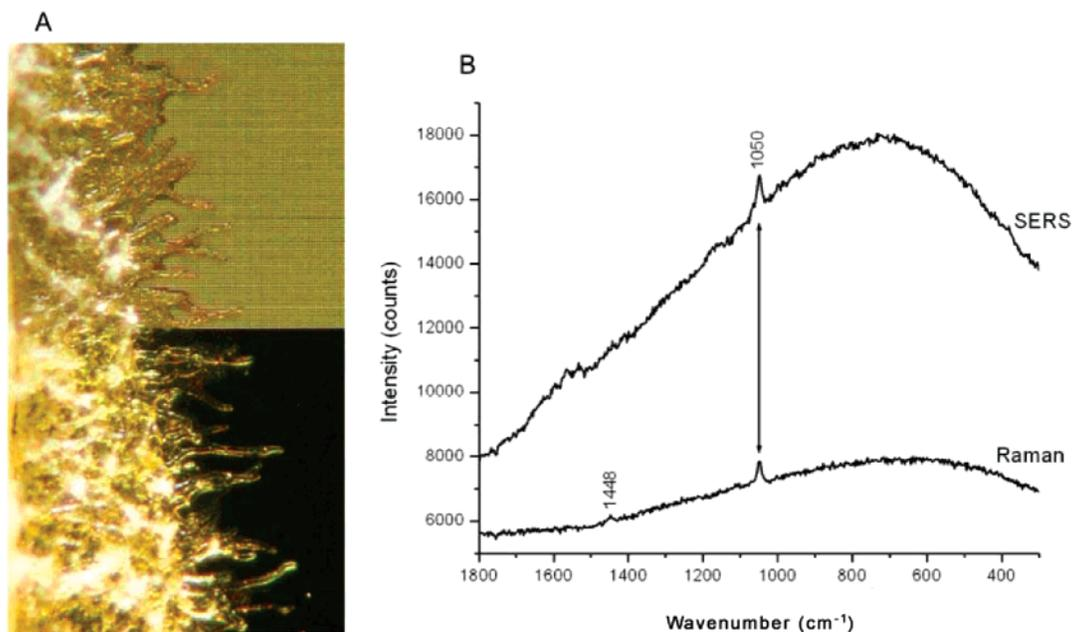
**Figure 1.** (A) Photoimage of the Klarite substrate showing the SERS-active pattern grid area (top half) and the smooth border (lower half). The fungi grown on the nanostructured region show no remarkable difference from those on the smooth area. (B) Representative Raman and SERS spectra of *A. nidulans*.
